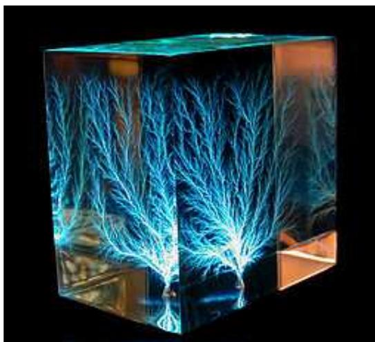
*Figure 1. 3D Lichtenberg “Lightning trees” in a block of clear acrylic.*
