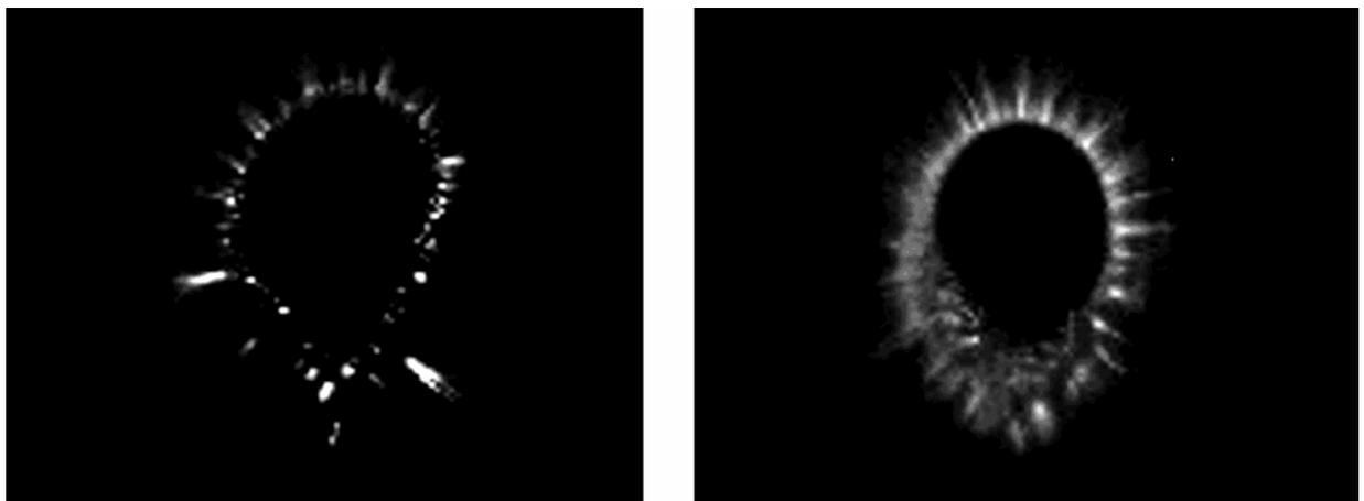
*Figure 5. Emission of a fingertip recorded without (left) and with (right) elastic insulator placed between the glass and finger.*
